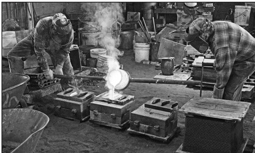
Over in the Uhrich Locomotive Works foundry, Marlin Uhrich (at right) and an assistant demonstrate pouring molten bronze to cast a new bearing for the Manitou & Pikes Peak Cog Railway. – Photo © 2014 Dave Schaaf.
